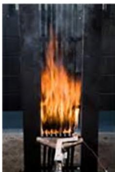
It is important to separate the fire performance of wire and cable from the LSZH label. Almost all modern cables are required to pass some type of flame test. Commonly UL 1666, UL1202, NFPA 262 and others. Nuclear power plants almost universally specify IEEE 1202, as cited in recent versions of IEEE 383 and IEEE 1682. Particularly in Ethernet electrical cables, and in fiber optic cables, LSZH cables meets the IEEE 1202, and the more severe UL 1666 riser and Canadian FT-4 requirements.
