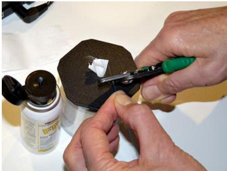
It is absolutely essential the bare fiber be perfectly clean before inserting into a ferrule during connectorization. Here the operator is preparing to clean with a high-quality lint-free wipe that does not contain any glues or cellulose. The cleaning fluid evaporates quickly and the canister cannot be refilled, which ensures the cleaning fluid will remain pure and uncontaminated.
