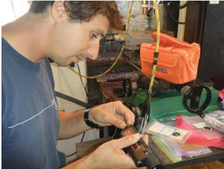
An essential element in the cleaning process is to inspect every endface, both sides, after cleaning. Here the operator has installed a new connector on the fiber-optic cable and is inspecting with a simple, handheld scope. Every technician who touches any fiber must be equipped with at least a low-power inspection scope.
