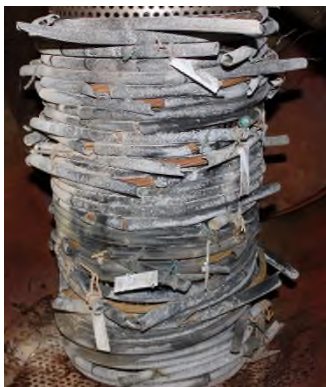
Figure 1. Conventional CSPE after LOCA and submersion
