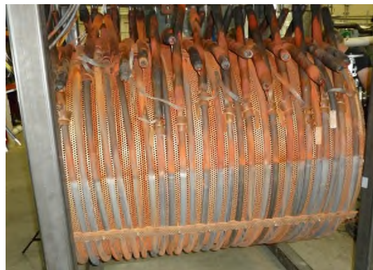
Figure 2. Ultrol 60+ after LOCA and submersion
